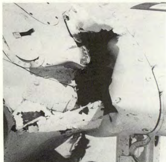
3. Turkey vulture strike to a T-37 wing root in the traffic pattern at Laughlin AFB, Texas. This photo graphically demonstrates the severe impact birds can have on our aircraft — even at T-37 airspeeds.
