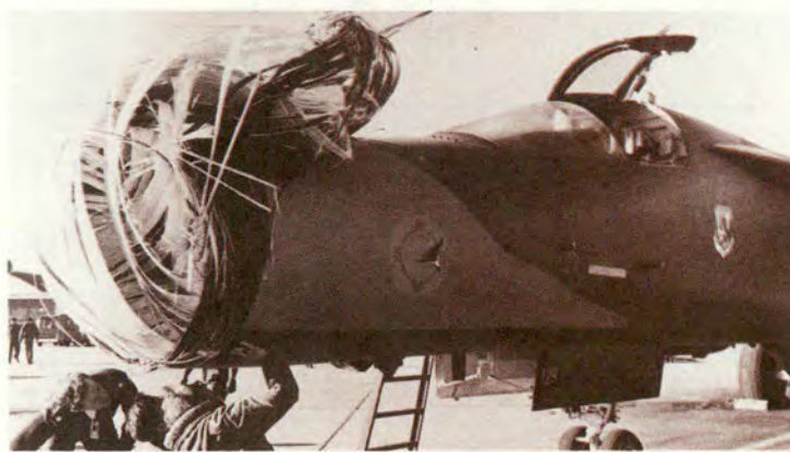
4. Red-tailed hawk strike to an F-111 at 475 knots low level from Cannon AFB, New Mexico. Not many pilots have flown while peering down the end of their own pitot tubes and lived to tell about it. An outstanding effort to set this one back on the ground.
